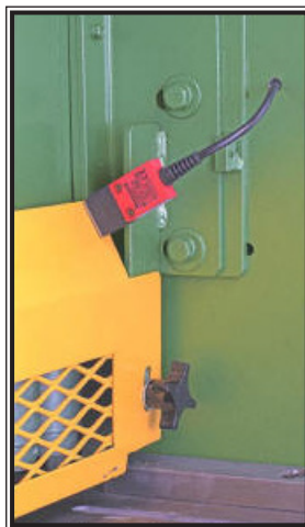
Safety Switch for Front Guard
