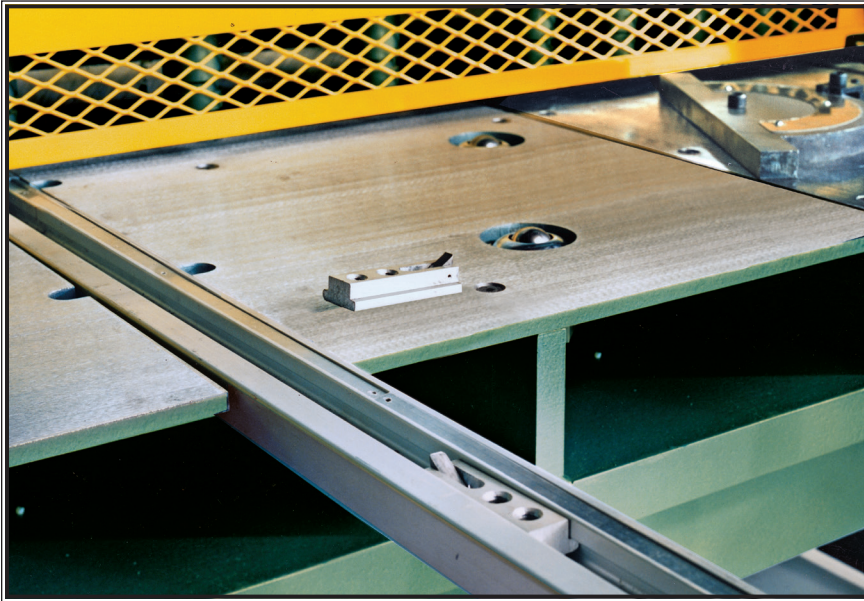
Segmented Table Top with Angle Gauge, Front Support Arms, Ball Transfers, Disappearing Stop and Inlaid Scale.
